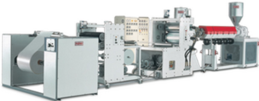
EVA Processing & Lamination Plant
